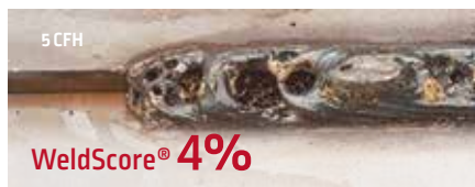
Unacceptable Weld – Low gas flow results in obvious porosity.
