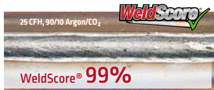
Acceptable Weld – Proper gas flow and coverage produces a good weld with no porosity.
