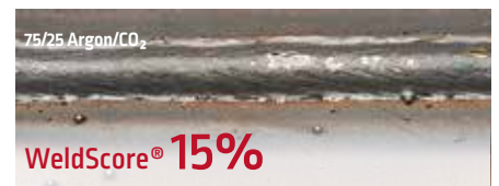
Unacceptable Weld – Incorrect gas mix yields higher spatter levels.
